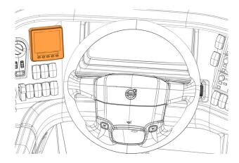
2. Retighten the screws fastening the display holder to the bracket. Apply a torque of **8 Nm ±1** (**71 lb-in ±9**). If a screw is damaged replace it by new screw 70368861.
