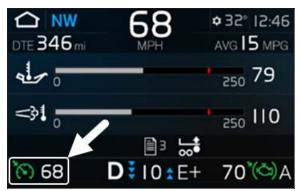
FIGURE 41: CRUISE CONTROL SET SPEED CONFIRMATION & CURRENT SET SPEED DISPLAYED IN THE SYSTEM STATUS ZONE
