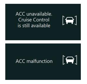
For the proper functioning of the system, the radar must be perfectly aligned and not blocked. If a radar fault condition is detected, one of the following pop-up messages will show in the DID.
