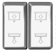
Press and hold the appropriate button to lower the left or right windshield sunshades. Press twice rapidly to raise or lower up to the end position.
