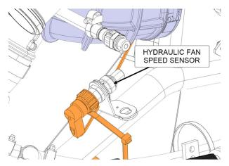
3) Cut cable-ties and remove the harness from its routing below the lower intercooler connection.
