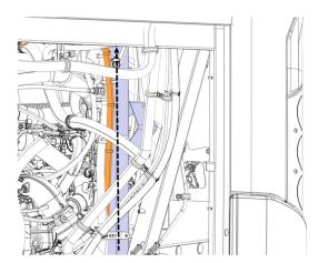
7) Use new cable ties 70312532 to secure the sensor harness along its new routing.
