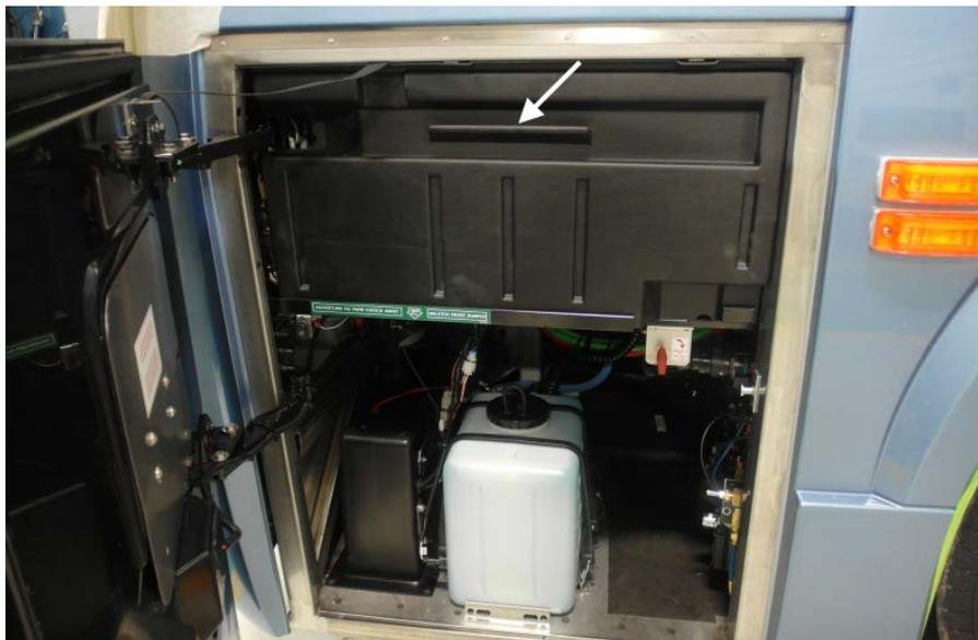
FRONT JUNCTION BOX PROTECTIVE PANEL (H3 VEHICLE SHOWN)
