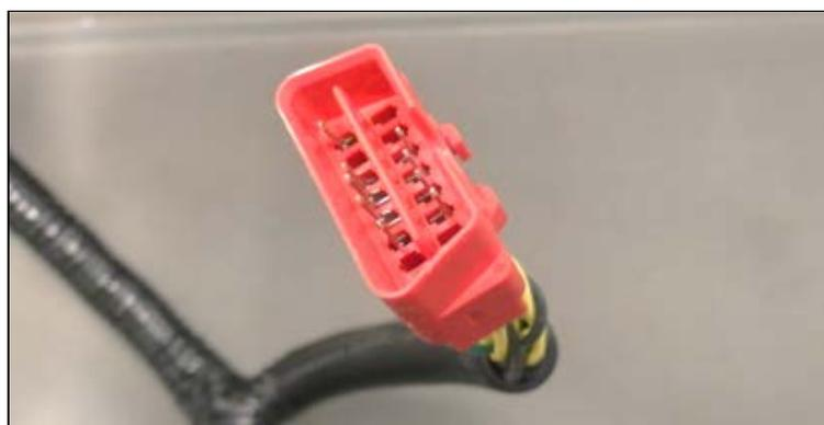
RED HARNESS CONNECTOR – TO VEHICLE OBD CONNECTOR
