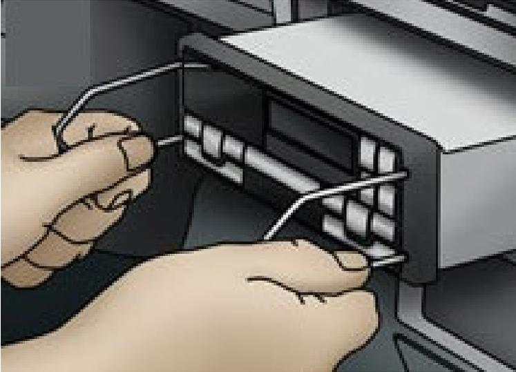
FIGURE 6: TYPICAL RADIO REMOVAL USING U-SHAPED TOOLS
