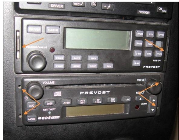
FIGURE 5: VERTICAL OPENINGS AND HOLES POSITION ON THE VSS AND RADIO UNIT FACES
