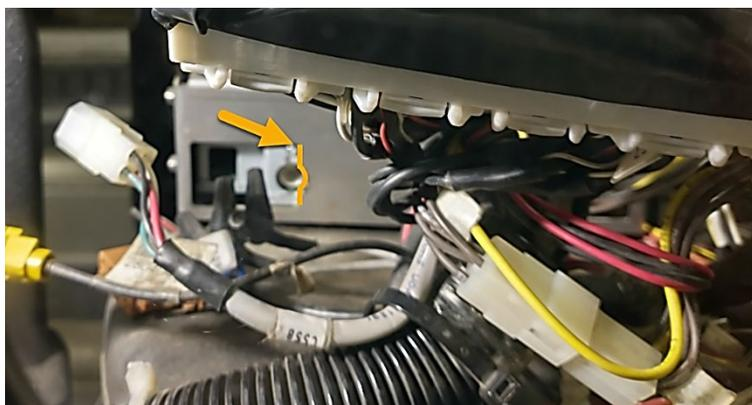
FIGURE 9: ENLARGED ANTENNA CONNECTOR OPENING
