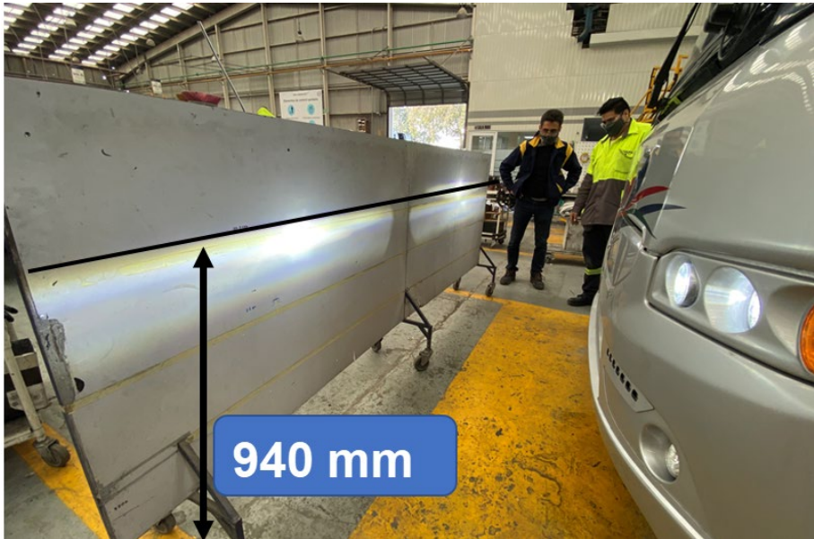
Figure 42: proper low beam height
