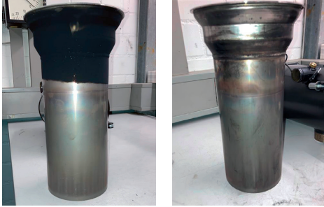
Combustion chamber before ... and after cleaning.
