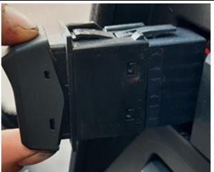
7. Press the connector tabs and unplug the switch from connector.
