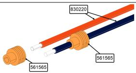
2. Crimp the terminals 561567 (2x) on the seals and on the wires of the lamp 830220.
