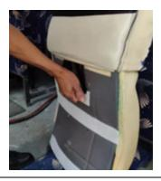
14. At the bottom of the backrest cover, attach the velcro.
