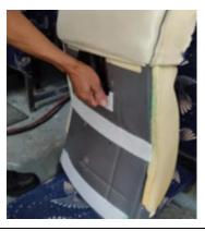
6. Remove the screws (4x per absorber) to remove the impact absorber.
