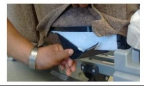
15. Reinstall the plastic guides with the screws (2x per guide).
