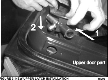
FIGURE 3: NEW UPPER LATCH INSTALLATION
