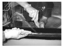
22. Make sure that lower edge of windshield section is well inserted in the bottom of rubber seal groove.
