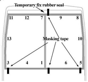
4. Make sure that rubber seal is properly positioned in the corners down to the bottom of the groove. Spray soapy water or "Clear Lube" Lubricant (800356) into the rubber seal groove on windshield side, especially in the corners.
