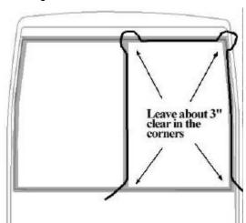
18. Spray some soapy water or "Clear Lube" Lubricant onto the windshield section.
