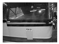
20. Rise up then tilt the windshield section, insert the first corner then the center of windshield.
