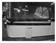
8. Rise up then tilt the windshield section, insert the first corner. Push windshield section towards the left, it must be well inserted in the bottom of rubber seal groove.
