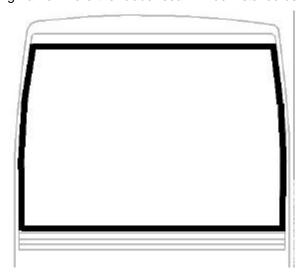
3. Install rubber seal, large side at bottom. Install as per following sequence and temporary fix seal in place using masking tape.
