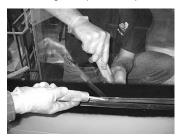
10. Make sure that lower edge of windshield section is well inserted into the bottom of rubber seal groove.
