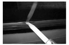
11. While maintaining a pressure onto the windshield section, gradually move the rubber seal lip aside to insert both sides of windshield section into the groove.
