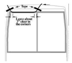
6. Spray some soapy water or "Clear Lube" Lubricant onto the windshield section.
