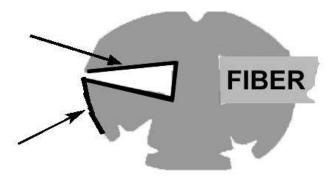
5. Insert a rope into the rubber seal groove to facilitate the installation of windshield R.H. side section.
