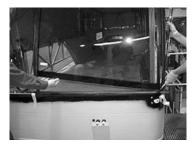
21. Insert lower part of windshield section using the plastic spatula. Push the windshield section in from the outside.
