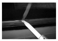
23. Maintain a pressure onto the windshield section. While pulling the rope, gradually move the rubber seal lip aside to insert both sides of windshield section into the groove.
