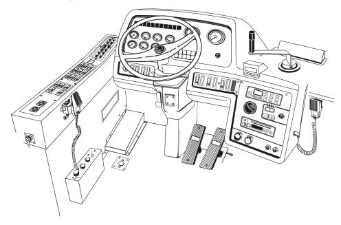
2. Push the lever down to unlock the steering column tilt and telescopic mechanism. Pull the steering wheel to maximum position then lock the mechanism.
