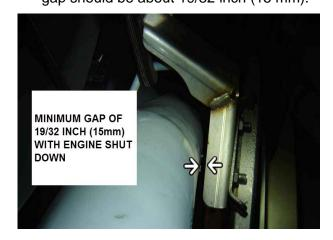
2) The picture below shows the area where interference between the 4-inch OD turbo outlet pipe and the close support bracket may be present.
