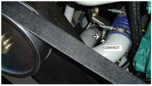
4) If evidence of rubbing is found, remove the support bracket and cut a part of the support bracket out as shown (as per image at left or at right as needed) and trim sharp edges.
