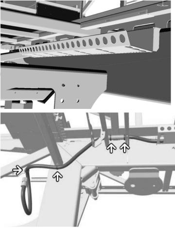
18. In engine compartment, use cable ties to secure hose as required.
