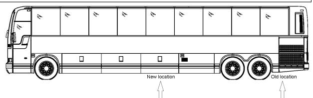
1. To access AFSS extinguisher cylinder, lift hinged rear fender, remove aft wheel and aft wheel arch liner.
