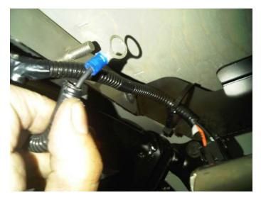
20. If no provision is available, route #068542 patch cable from the original cylinder location in the engine compartment up to the third baggage compartment. Routing of the patch cable follows usual harness routing in vehicle as shown in view below.
