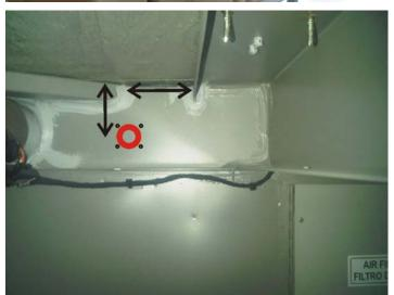
10. Install Extinguisher Cylinder structural support road side and curb side #406562 & #406563. Refer to drawing D400463 for positioning.
