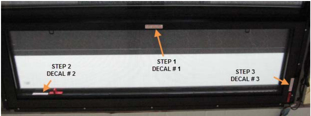
Fig.3 Awning window emergency exit opening sequence.
