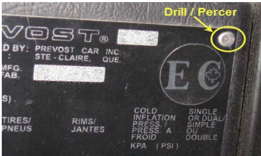
Fig.7 Rivets to be removed (4X).
