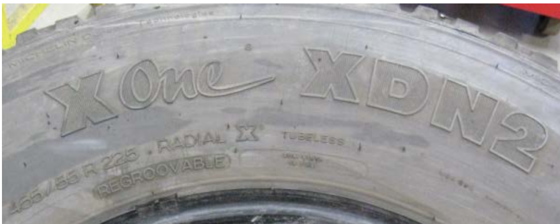
Fig.4 OEM Michelin "X One Super Single" wide base tire (455/55 R22.5).
