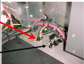
Using electric tape, insulate the 2 largest gage wires. Make sure the ring terminals do not touch each others and the vehicle body.
