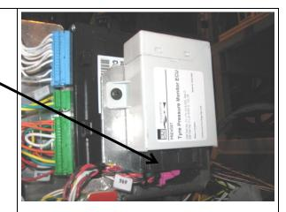
Disconnect connector A 83 under Volvo Link module
