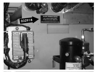
2. Affix new belt routing decal #012698 on the left engine compartment door as shown on picture, replacing former decal #019095. Do not leave decal #019095 on the door if it remains visible.
