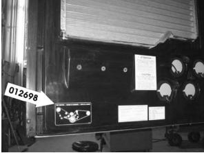
3. Affix new oil specification decal #012702 as shown on picture, replacing former decal #012399(eng/fr) or #012400 (eng/esp). Do not leave the existing decal in the engine compartment if it remains visible.
