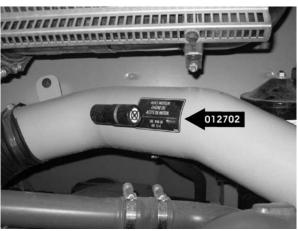
4. Affix new coolant specification decal #053597 as shown on picture, replacing former decal #0534787(eng/fr) or #053488(eng/esp). Do not leave the existing decal in the engine compartment if it remains visible.
