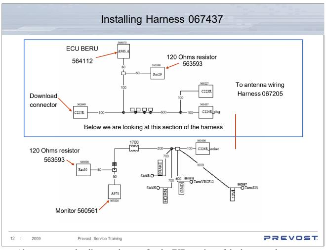
Above you see the diagram lay out for the FJB portion of the harness, the harness can be split at C224 for ease of instillation and inspection. Below is the ECU & antenna portion split harness.
