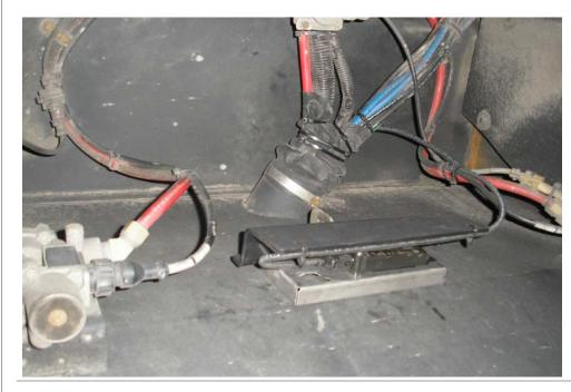
From the spare tire Compartment route C100 through the tube to the front axle area.
