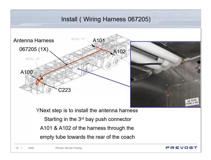
Open all the bays on the drivers side of the coach, feed C-102 & C-101 through the open tube as seen in the photo above, pull enough of the harness through to the last bay to reach the tag axle area. Then route C-223& A-100 between the 2 PVC pipes all the way to the front bay. You can use cable ties to support the harness but do not secure them at this time
