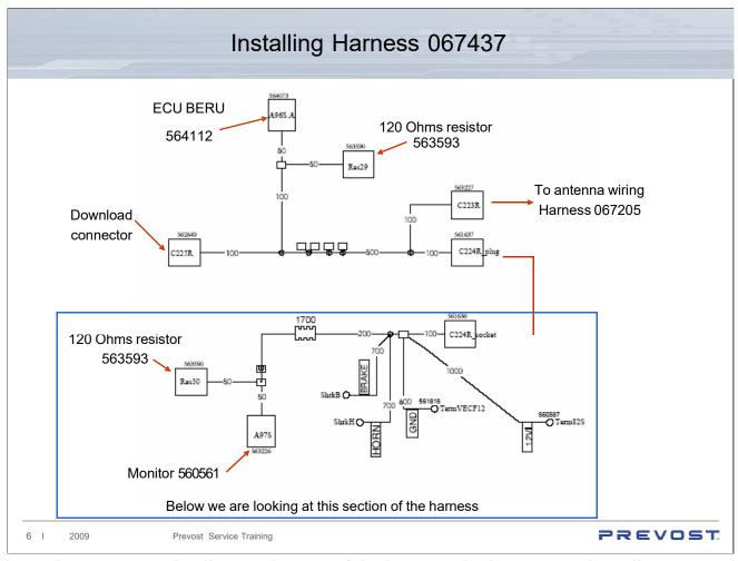
Above you see the diagram lay out of the harness, the harness can be split at C224 for ease of instillation and inspection. Below is the split harness.
