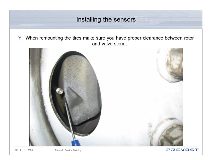
Make sure to respect the proper torque and position of the valve stem offset when remounting the tires on the drive.
