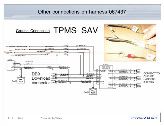
Next we connect the <u>Electronic ground</u>, wires are labeled as shown above. The wire that is labeled GND with the ring terminal shown above should be connected to the electronic ground located in the FJB as shown below
