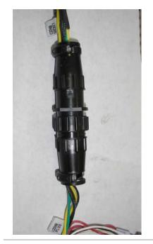
Move socket terminal from 7 to 5 to match pin terminal
