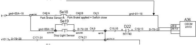
For non Multiplex you will need to connect the park brake signal wire to terminal 87 of the R-5 Relay in the FJB. This will require a terminal part # 561181.
