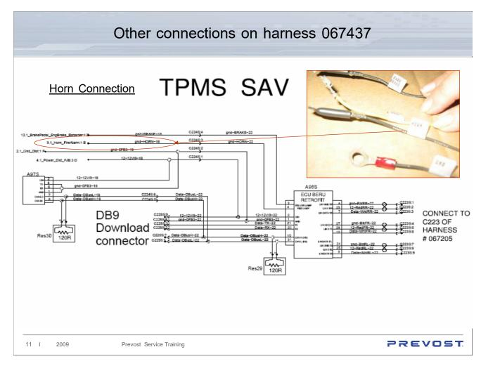
Next we connect the <u>horn</u>. circuit, connections are labeled as shown above. For Multiplex coaches we connect the <u>horn wire</u> to circuit 0-69 at module A45 J1:10
