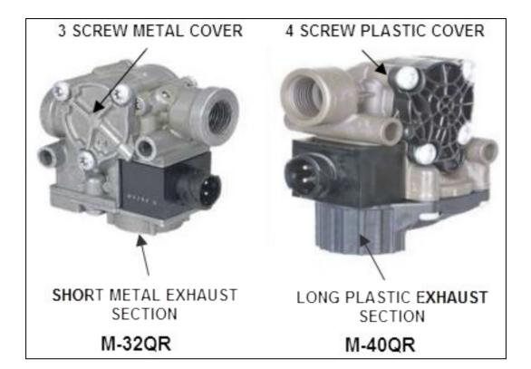
Modulator valve model can be easily identified by their different side cover and exhaust section.
