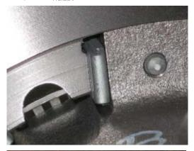
16. Insert all of the spring elements with their screws and tighten by hand. Fit each spring elements with its tang pointing to the friction ring (see arrow).
