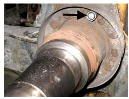
11. Remove the round metal sheet protecting the sensor and toothed wheel (identified with arrow). This part won't fit with the use of splined disc.
