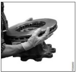
14. Apply anti-seize compound (Permatex Copper Anti-Seize Lubricant) on both sides of intermediate elements (item 4).
