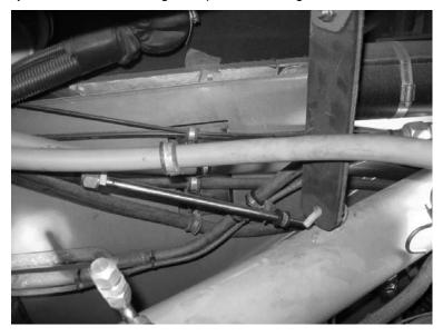
8. Connect power steering hose to noise reducer fitting.
