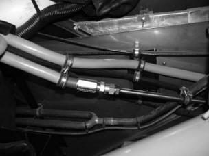
10. Secure power steering hose using clamps, retainers and cable ties.
