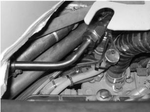
7. Secure power steering hose using clamps, retainers and cable ties.
