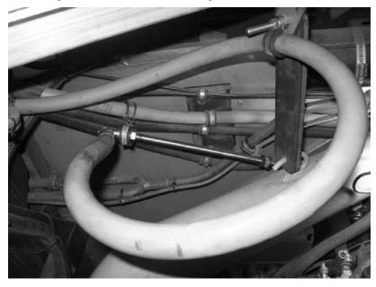
9. Instead of using previously removed elbow fitting, you can use supplied fitting (501005) to connect hose to noise reducer. To do so, from the engine access hatch, cut hose and fasten fitting (501005).
