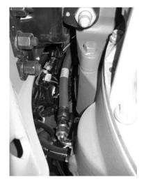
6. Connect power steering hose to noise reducer fitting.
