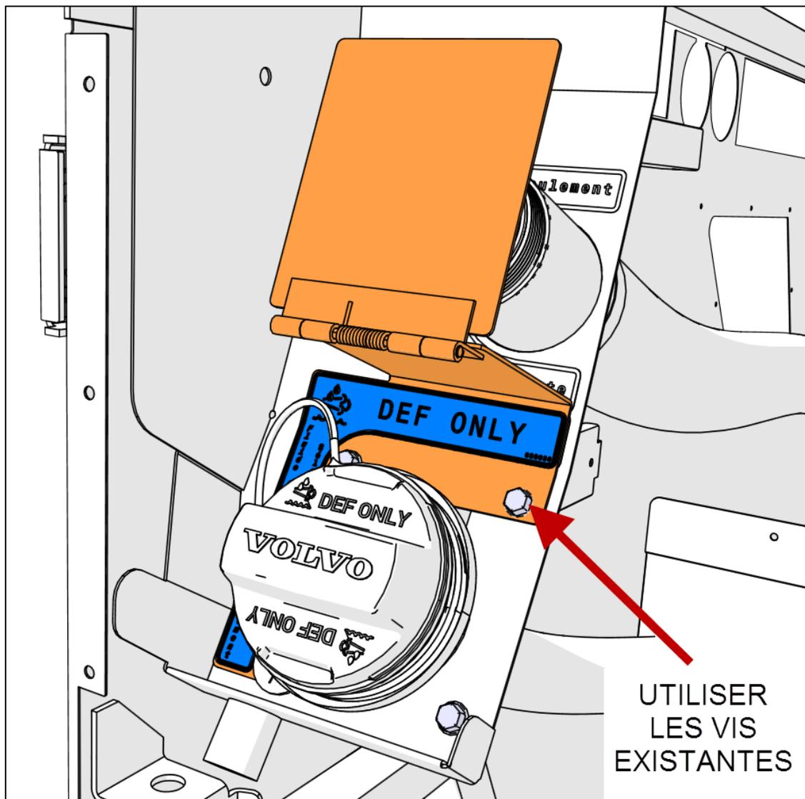
FIGURE 1: MODÈLES H3 INSTALLATION DE LA TRAPPE
