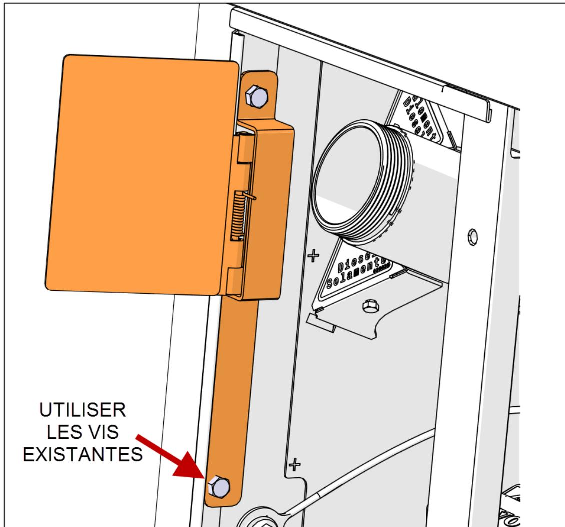
FIGURE 3: MODÈLES X3 SANS SERRURE INSTALLATION DE LA TRAPPE
