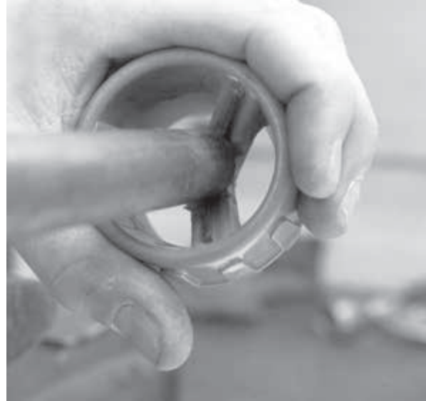
FIGURE 14: DEBURR THE TUBE END - OUTER
