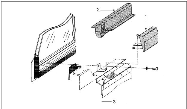
FIGURE 3: VENTILATION GRILLE (3) AND RELATED COMPONENTS
