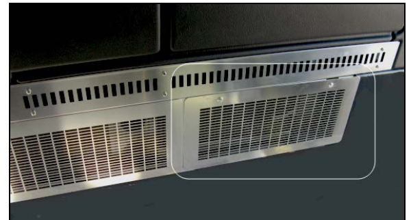
ACCESS TO DRIVER'S HVAC UNIT AIR FILTERS
