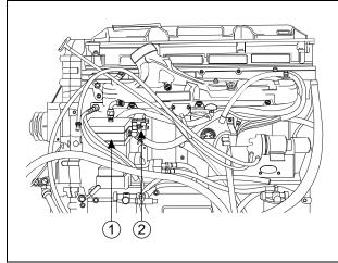
FIGURE 1 : ① AIR COMPRESSOR, ② AIR COMPRESSOR GOVERNOR
