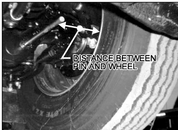
FIGURE 4: POSITION PIN INSTALLATION
