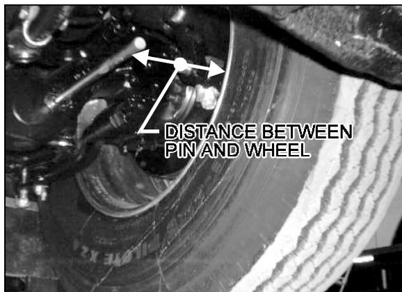
FIGURE 4: POSITION PIN INSTALLATION
