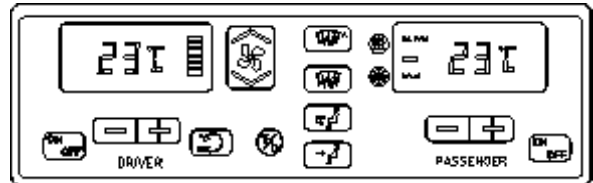
FIGURE 5: CENTRAL HVAC SYSTEM CONTROL MODULE
