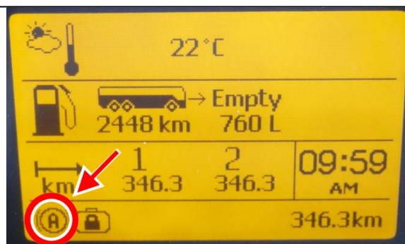
FIGURE 42 : PROCEDURE COMPLETED SUCCESSFULLY, THE PICTOGRAM **(A)** APPEARS IN THE DID STATUS LINE
