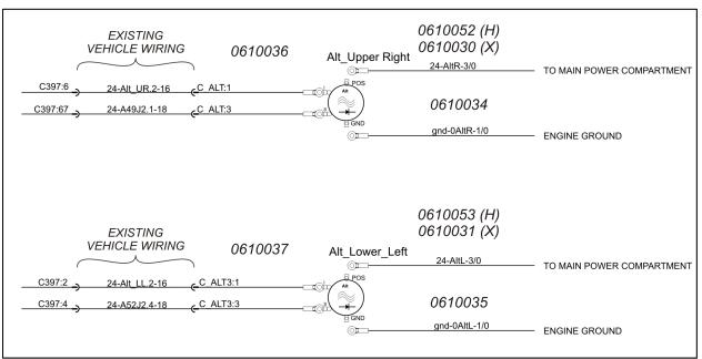
FIGURE 1: ALTERNATOR CONNECTIONS W/ HARNESS NUMBERS
