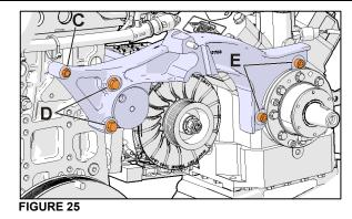
28. Tighten compressor base mounting bolts to 82 lb-ft
