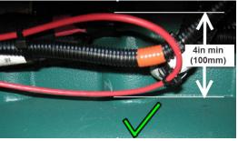
LTD is not a flexible harness. Avoid tight bends and kinks which could short circuit the LTD. Loops must hace a minimum radii of 4 inches (100 mm)
