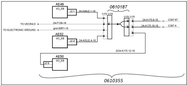
FIGURE 3: BOOST REGULATOR / HARNESS 0610355 CONNECTIONS IN MAIN POWER COMPARTMENT
