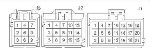
**FIGURE 4: IOEB PINOUT**
