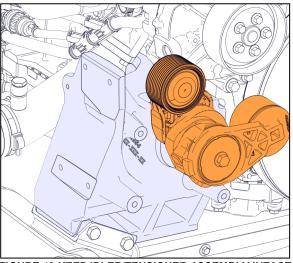
FIGURE 48:KEEP IDLER/TENSIONER ASSEMBLY INTACT
