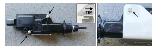
7. Install the new actuator, adaptor bracket & harness assembly to the vehicle support using the supplied M4 hardware (5001036 screws, 502636 washers & 502524 nuts). If the support was removed from the vehicle, reinstall the complete assembly.
