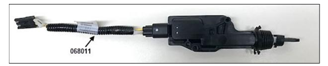
Secure the new 2800049 actuator to the 2810380 adaptor bracket (Use supplied 5001100 screws, 500437 washers & 5001408 nuts). The tip of the actuator must be mounted toward the "straight" (90deg angle) part of the adaptor.
