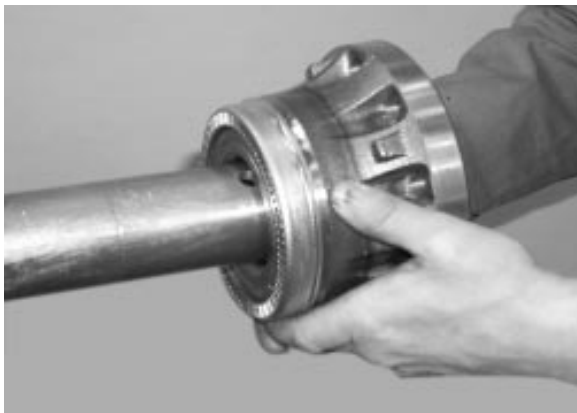
FIGURE 11: SLIP UNITIZED HUB BEARING OVER SPINDLE
