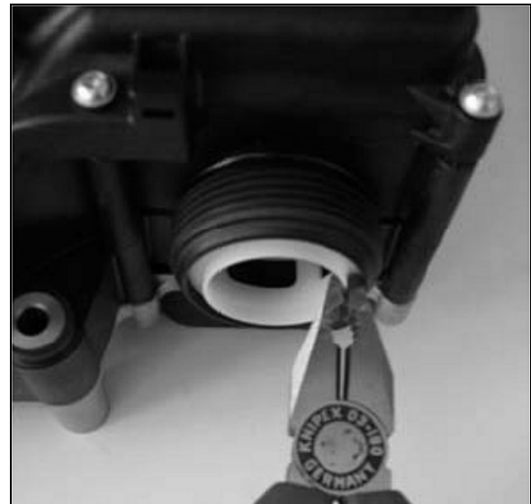
FIGURE 12 : PUMP ASSEMBLY FILTER ELEMENT
