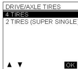
Pressing the up down arrow when the number of tires is highlighted allows flipping the number to 2 or 4 which are the only valid choices.
