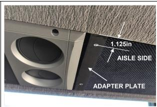
2. Using the adapter plate as a template, drill two 5/16in holes in the overhead panel.
