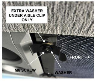
Clip in place the scissor screen and check for correct adjustment. The screen should deploy and retract easily and should not contact the side window or lateral sun shade. Adjust laterally as required.
