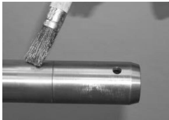
FIGURE 18: APPLY GLEITMO 805 GREASE
