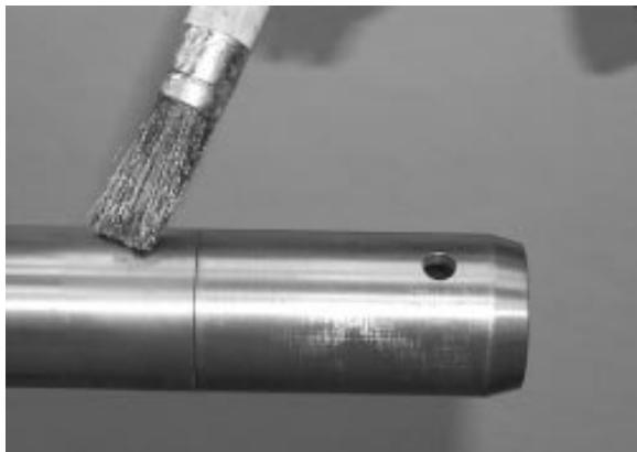
FIGURE 9: APPLY GLEITMO 805 GREASE
