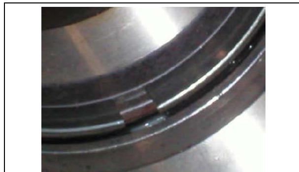
5. Clean thrust washer both sides and hub nut using EFX degreaser.
