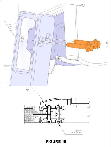
19. Present the Vertical support #21693935 in order to transfer the fixation holes to the partition wall pillar.
