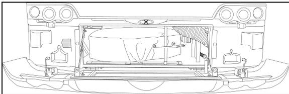
**FIGURE 11: X3 SERIES SPARE WHEEL COMPARTMENT**
