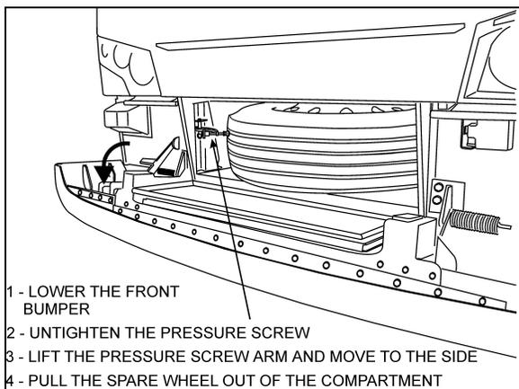
**FIGURE 13: H3 SERIES SPARE WHEEL AND TIRE**
