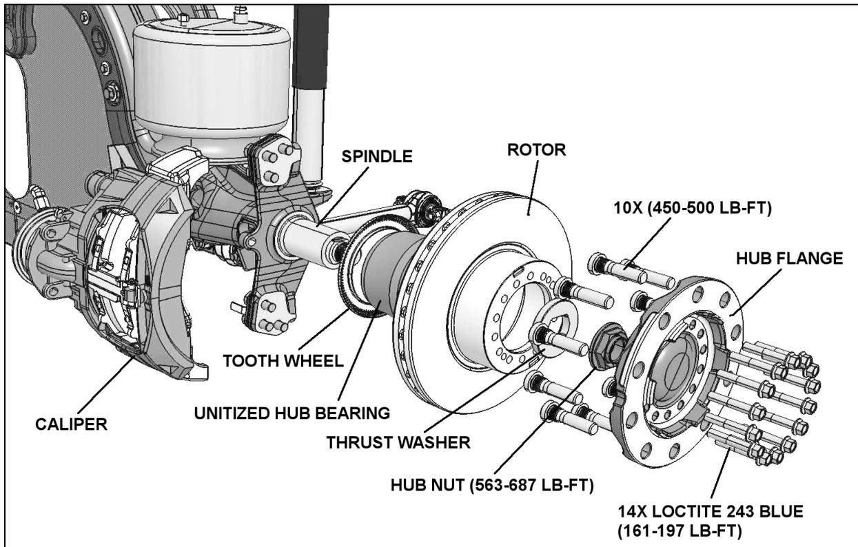
FIGURE 8: FRONT &amp; TAG AXLE HUB AND ROTOR ASSEMBLY
