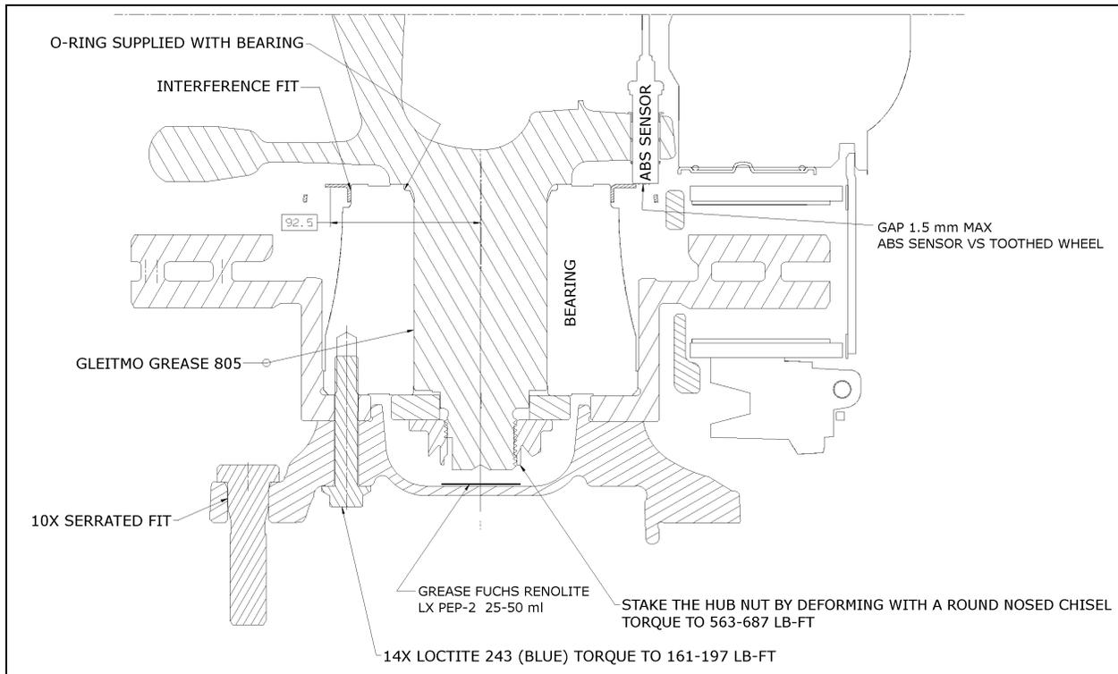
**FIGURE 7: FRONT & TAG AXLE WHEEL HUB**
