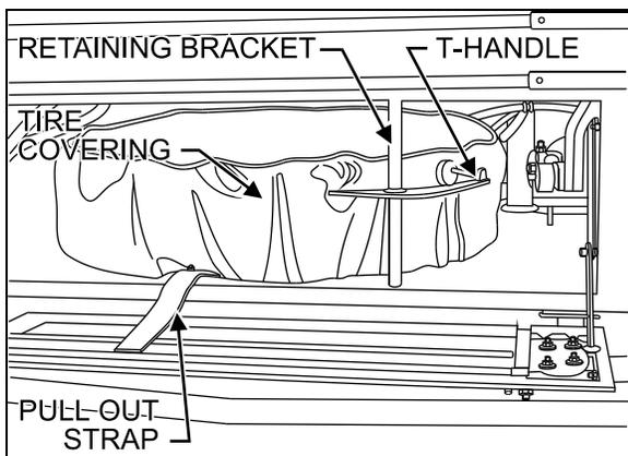
**FIGURE 12: X3 SERIES SPARE WHEEL AND TIRE**
