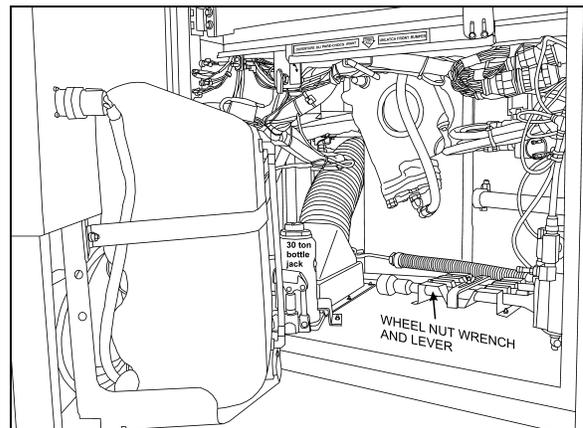
**FIGURE 14: FRONT SERVICE COMPARTMENT OF A X3 SERIES VEHICLE**
