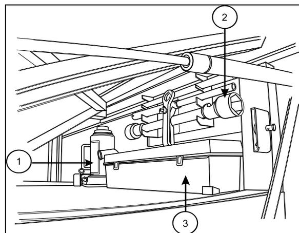
**Figure 15: forward compartment of H3 series vehicle with jack, wrench and reflector kit.**
