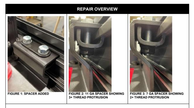
In some instances, the two bolts used to clamp the rear wall mounting brackets on the 2096 transverse recliners to the wall track of a Prevost bus may slightly contact the seat frame bracket.
