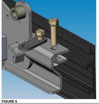
3. Remove and replace Nord-Lock washer onto new back bolt, swing spacer into position and reinsert new bolt into back position by FINGER TIGHTENING into the nut of U-bracket.
