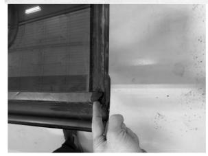
6. In case of using **22040451** GASKET AS RAW MATERIAL (per meter), make a correct window seal for the frame, cut the edges at 45°.
