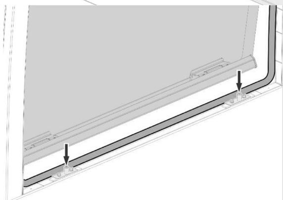
12. Adjust the lock mechanism from the inside if necessary.
