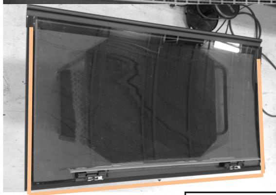
9. Measure and apply double sided **ADHESIVE TAPE 70363904**, subsequently neoprene trim **21331618 MOLDING, EMERGENCY WINDOW (EPDM)** on the sides.
