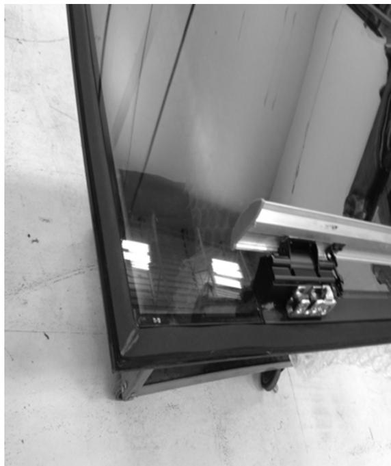
Check the correct sealing of the window, on the inside all around. If necessary, measure and install more ADHESIVE TAPE **70363904**, subsequently neoprene trim **21331618 MOLDING, EMERGENCY WINDOW (EPDM)** on the window where the seal is not achieved.
