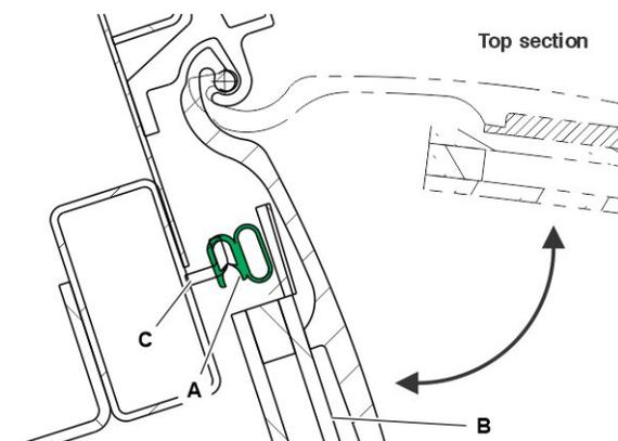
15. Only if necessary, measure and apply double sided ADHESIVE TAPE **70363904**, subsequently neoprene trim **21331618** MOLDING, EMERGENCY WINDOW (EPDM).
