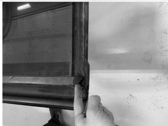
6. Route the **23620744** Gasket inserting it on the metal lip frame. Start at the bottom corner of the window's frame, radius at the corners as small and smooth as possible.
