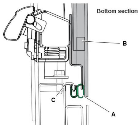
17. If necessary, measure and apply double sided ADHESIVE TAPE **70363904**, subsequently neoprene trim **21331618 MOLDING, EMERGENCY WINDOW (EPDM)** on the bottom.
