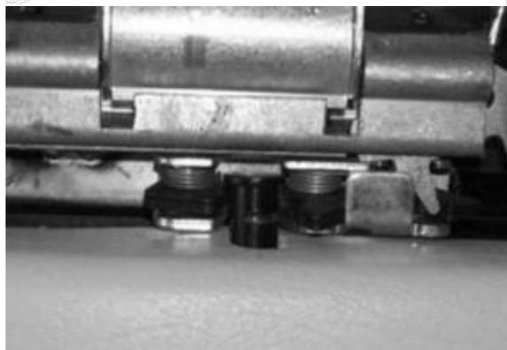
13. Loosen the lock screws and slide forward or backward as needed, later apply torque to screws
