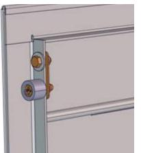
32. Secure the new **2810358** latch plate, **2810232** strike plate & **2810360** backplate to the vehicle using four **502622** screws & four **5002015** washers.
