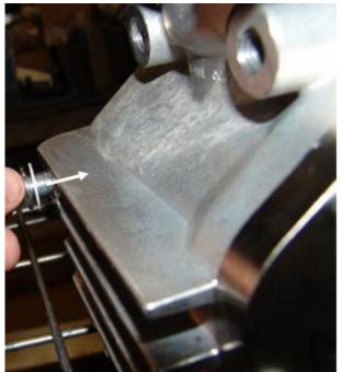
Remove the breather/dipstick from the top of the gearbox and pour 22 oz (650 mL) of 75w-90 synthetic gear oil into the gearbox.
