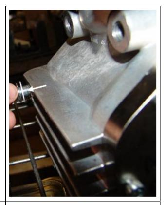
Before reinserting the plug wipe the magnetic portion of the plug off to remove any contaminants. (The magnetic portion is the part that gets inserted into the gearbox).
