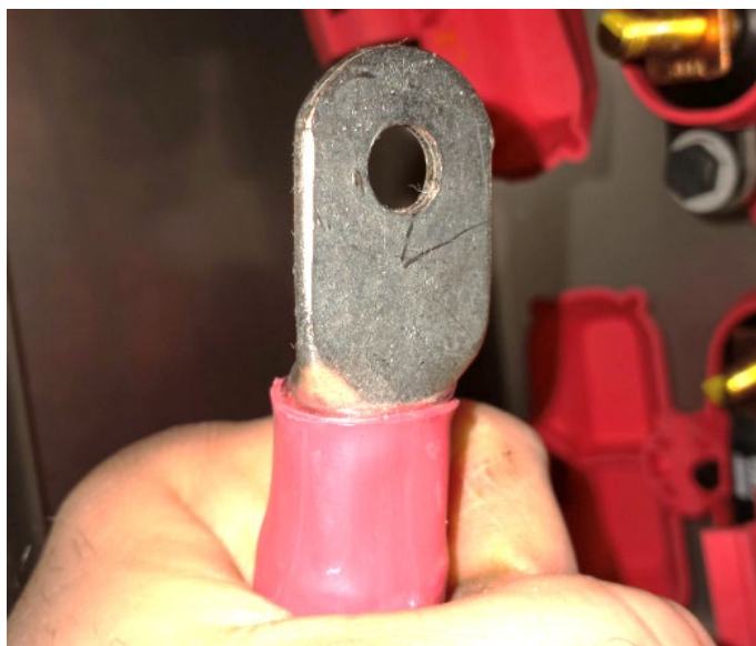
Figure 3: cable lug in good condition, no heat effects
