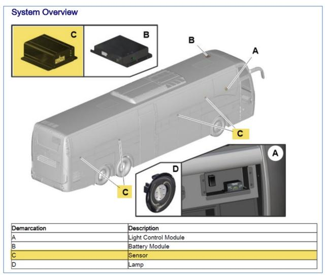
Figure 1: sensor location item C, 4 sensors
