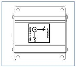
Figure 9: sensor with axes decal
