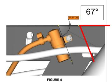
6. Tighten the screw that hold the clamp.
