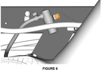
Writer: MG/OL <QF7720955 rev 7> 7. Verify the air filter indicator is visible.
