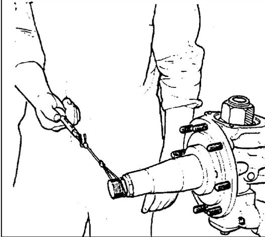
**FIGURE 2: METHOD OF CHECKING SWIVEL BEARING ADJUSTMENT** 10017
