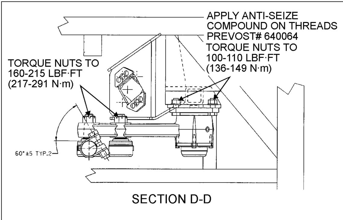
FIGURE 5: CLAMP POSITIONING
