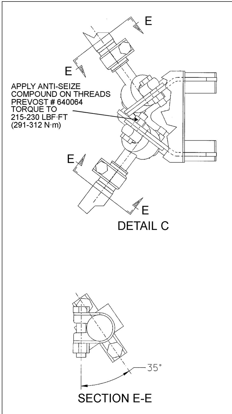
FIGURE 6: CLAMPS POSITIONING
