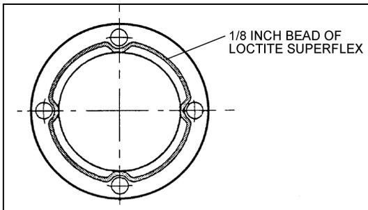
**FIGURE 7: HUB CAP AND HUB MATING FACES**
