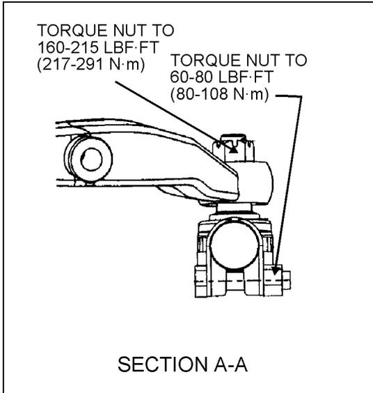
FIGURE 3: CLAMP POSITIONING
