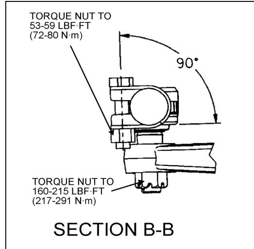
FIGURE 4: CLAMP POSITIONING
