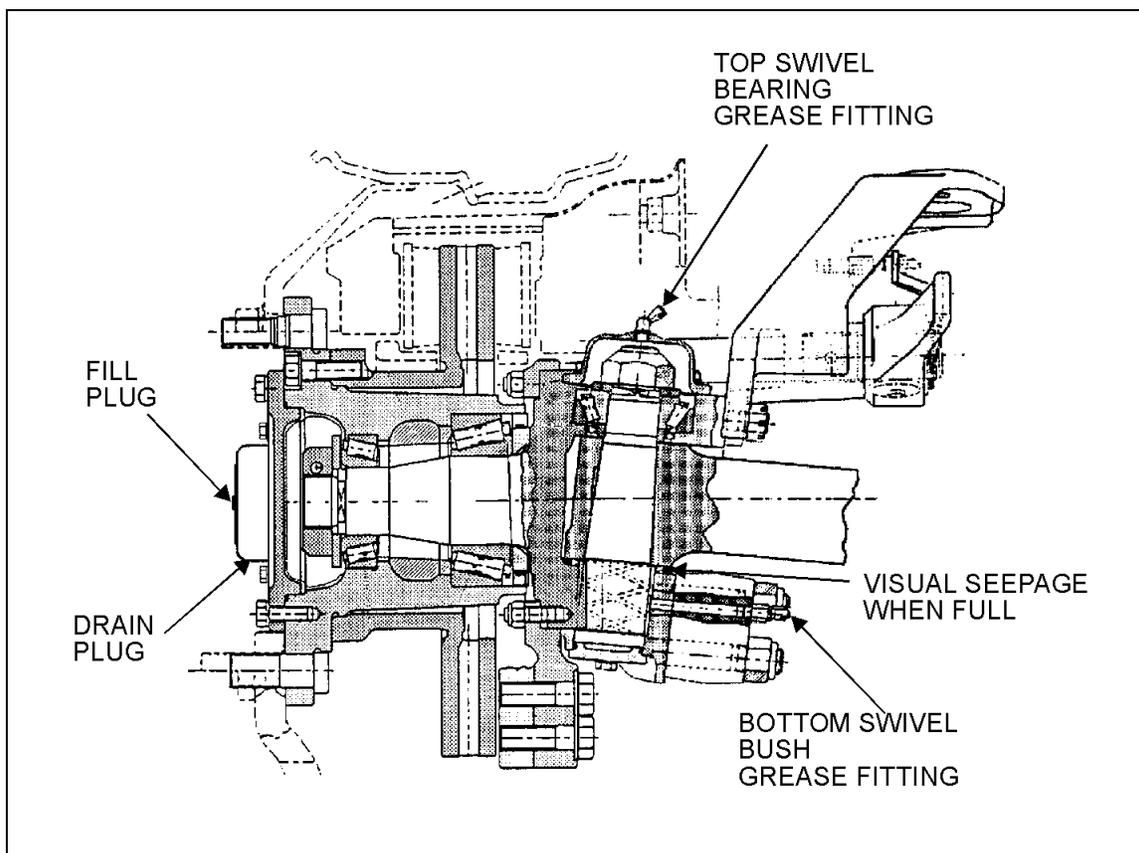
FIGURE 1: SWIVEL GREASING POINTS AND HUB OIL LUBRICATION
