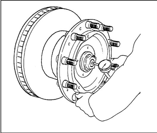
**FIGURE 6: TO ADJUST HUB 'END FLOAT'** 10021
