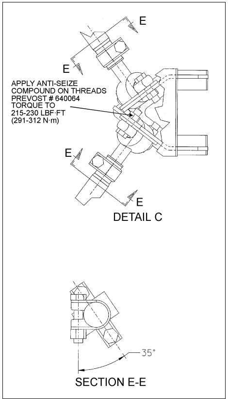
FIGURE 6: CLAMPS POSITIONING
