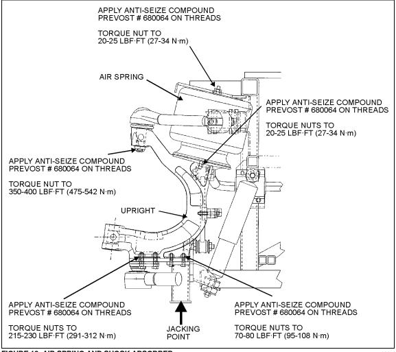
FIGURE 18: AIR SPRING AND SHOCK ABSORBER
