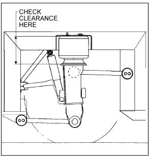
FIGURE 12: TYPICAL AIR SPRING CLEARANCE
