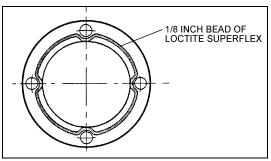
FIGURE 7: HUB CAP AND HUB MATING FACES
