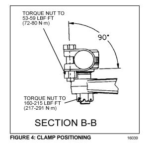
FIGURE 3: CLAMP POSITIONING
