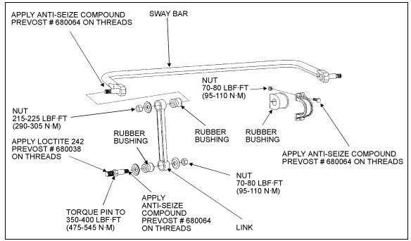
FIGURE 20: SWAY BAR (FRONT SUSPENSION)
