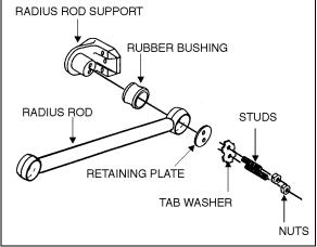
FIGURE 6: TYPICAL RADIUS ROD SETUP
