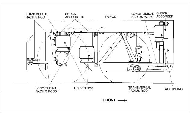
FIGURE 2: REAR SUSPENSION COMPONENTS
