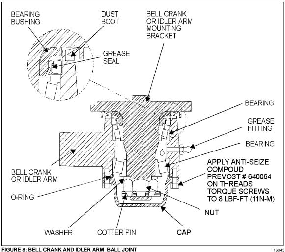
FIGURE 8: BELL CRANK AND IDLER ARM BALL JOINT
