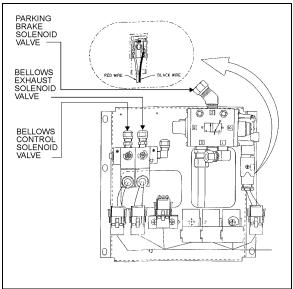
FIGURE 14: KNEELING/HI-BUOY PANEL (STEERING COMPARTMENT) 16031
