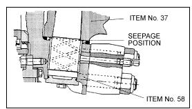
FIGURE 5: PART SECTION THRO' BOTTOM OF SWIVEL SHOWING GREASE SEEPAGE POSITION WHEN FULL 10020
