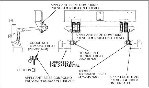
FIGURE 21: SWAY BAR (DRIVE AXLE)
