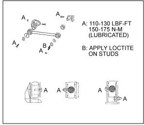
**FIGURE 9: RADIUS ROD INSTALLATION**
