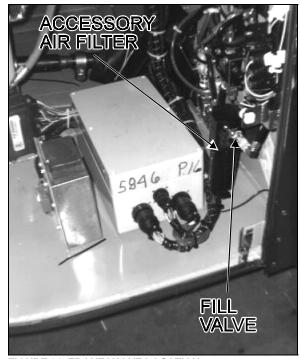
**FIGURE 31: FRONT VALVE LOCATION**
