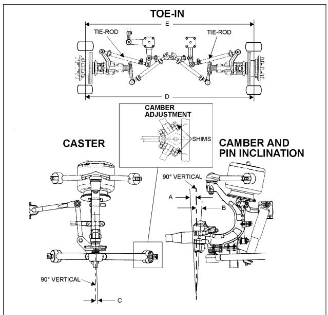
FIGURE 16: FRONT END ALIGNMENT DIAGRAM
