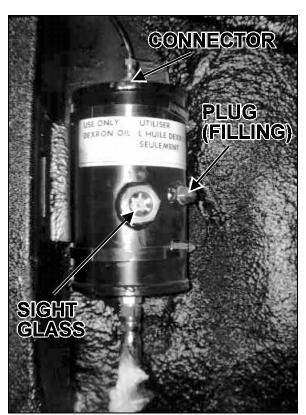
FIGURE 17: DRIVE AXLE STABILIZER RESERVOIR 16034
