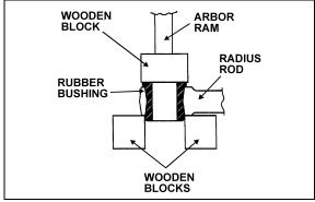
FIGURE 8: RADIUS ROD BUSHING INSTALLATION 16012
