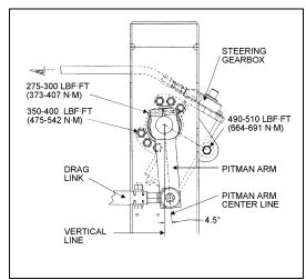
FIGURE 7: PITMAN ARM ALIGNMENT
