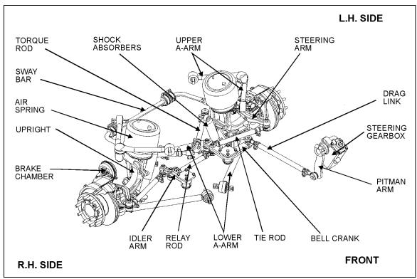
FIGURE 1: SUSPENSION AND STEERING LINKAGE
