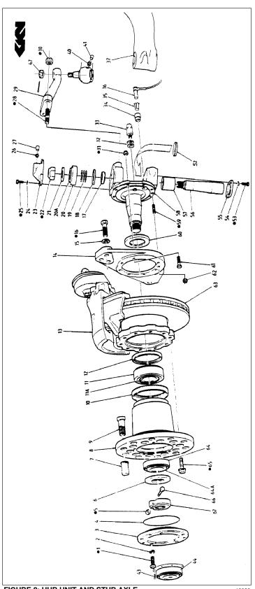
FIGURE 8: HUB UNIT AND STUB AXLE
