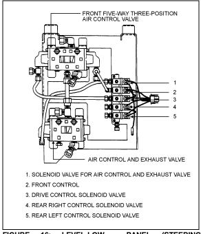
FIGURE 16: LEVEL-LOW COMPARTMENT)
