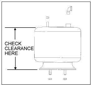
FIGURE 23: TYPICAL AIR SPRING CLEARANCE
