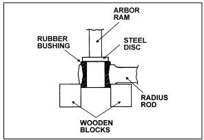
FIGURE 7: RADIUS ROD BUSHING REMOVAL
