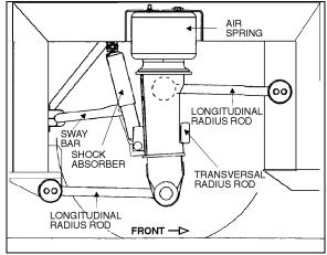
FIGURE 1: FRONT SUSPENSION COMPONENTS
