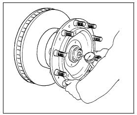
FIGURE 6: TO ADJUST HUB 'END FLOAT'
