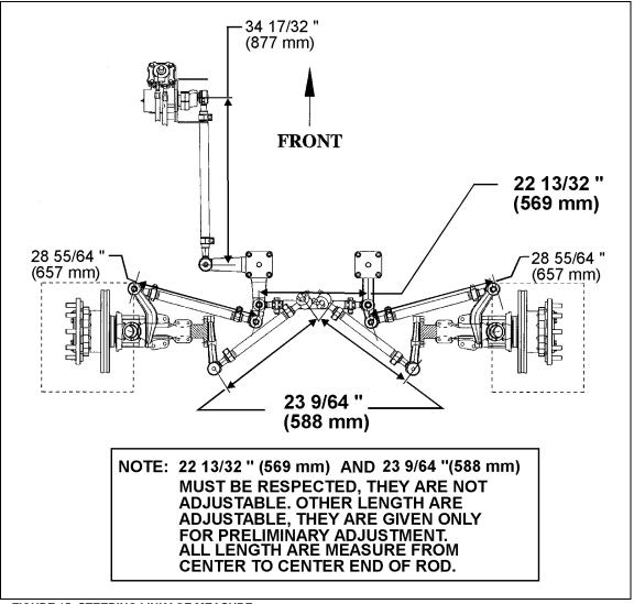
FIGURE 15: STEERING LINKAGE MEASURE
