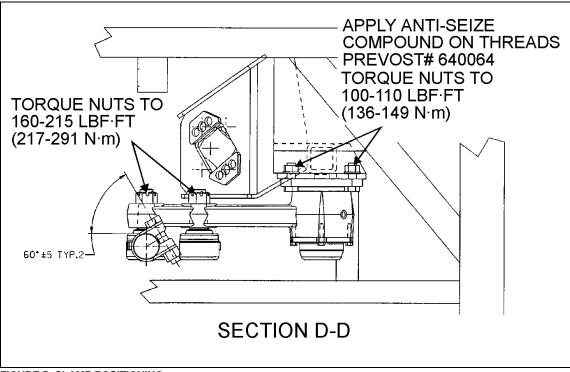
FIGURE 5: CLAMP POSITIONING
